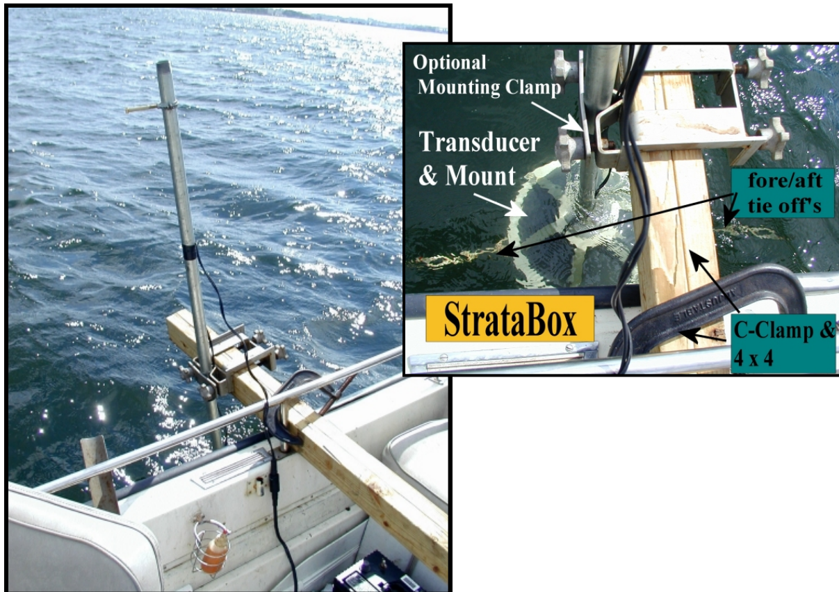
Figure 2-4 Over The Side Transducer Mounting
